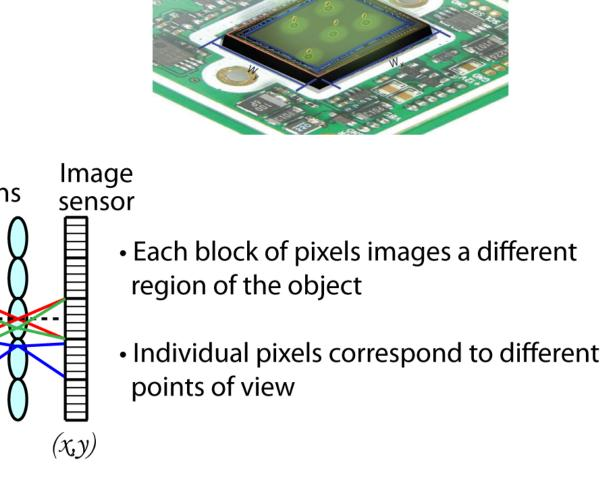
Pixel-level sensor augmentation for compact multi-modality
